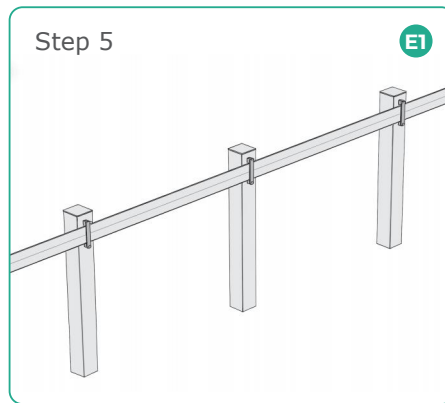
After finishing, installing the rest Rail Brackets with Flexible Rail.
